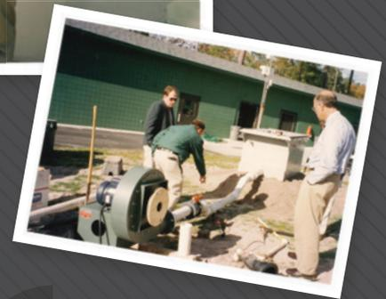
*This first test was to determine that air would move easily through the soil mix of a USGA green and also that the pressure blower was capable of providing enough air.*
